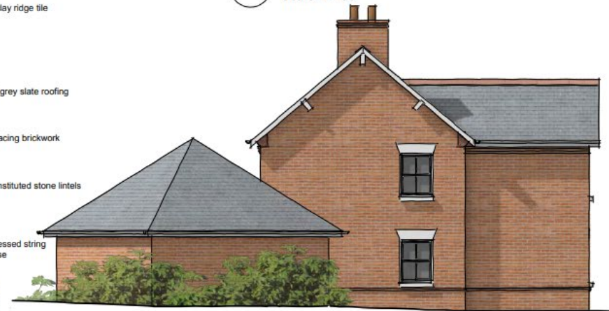
5 Special House Type 3 East Elevation Scale: 1:100
