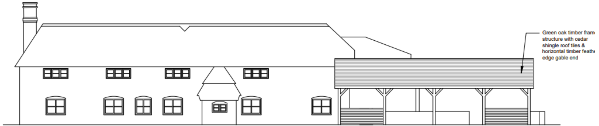
NORTH ELEVATION SCALE 1:100
